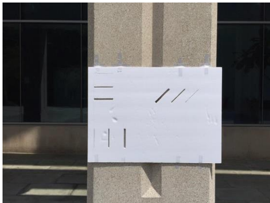
(a). Foam board for cracks simulation.
