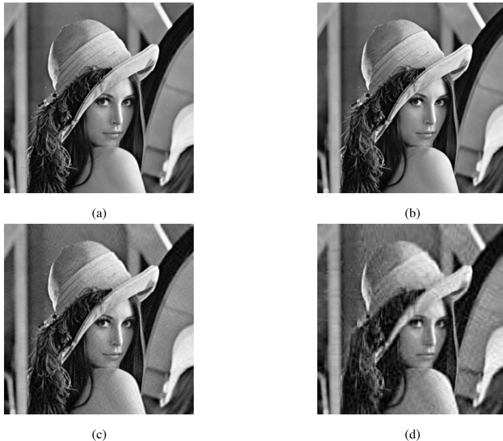
Fig. 2: Lena's image of size 256x256 reconstructed by eq. (4) (a) original Lena image (b)reconstructed using 128 \sigma (c) reconstructed using 64 \sigma (d) reconstructed using 32 \sigma
